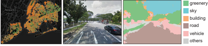
Fig. 3. Illustration of data preprocessing: sampling locations in New York City are generated from OpenStreetMap (left), a street view image is collected from Google Street View (center), and the image pixels are classified into six features using SegNet (right).
