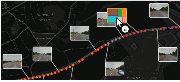
Fig. 6. Street Map View provides an overview of all street views along a street as colored points, and highlights images on two sides of the street. (a) A tree map showing the feature composition of an image will pop up when the mouse pointer is hovered over the image.
